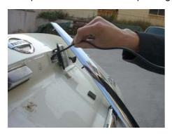
4. Make the power cable of camera through the light hole of license plate, fix up the transmitter board on the surface of armor plate of the later cover(Notice:if the transmitter put in the interbeded of will affect the receive quality)
