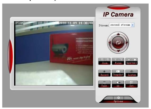
After logged on the device, monitor picture is displayed on the left side of the screen, and the right side is the panel where you can implement the basic operations for the device.
