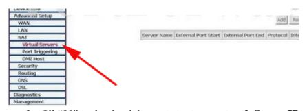
3. fill "80" under the right **port start** or **port end**, **Server IP address** fill "192.168.1.50", protocol select "TCP/UDP"OR" "TCP", finally don't forget click under ""save/apply"
