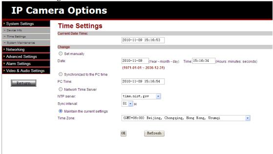
You can set the time manually, or synchronize time with the PC or NTP server.
