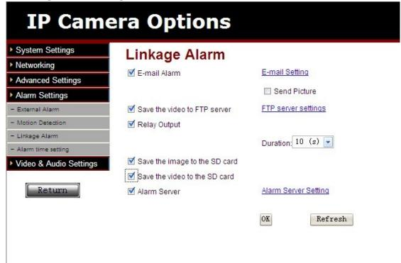
Here you can set the linkage alarm actions ,such as sending the photo to specified email,saving photo and video to SD card or specified FTP server.,
