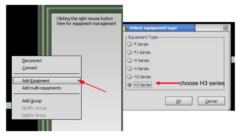
When finish adding camera, if needs to change other settings, please select the camera, and click the right key to choose equipment setting and then set the parameters, also users can click one monitor screen, then click to set the camera. The information need to be finished include the basic information, equipment parameters, alarm, record, action plans, additional information. The following text we will give you a more detailed explanation.
