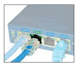
If connecting the LAN successfully ,the green LED light on the RJ45 interface will be on .If there are datas transmissons on the LAN, orange LED light will flash.
