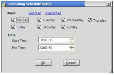
When device needs recording, first enter setting configuration to configure Enable Record: Only when "Enable Record" is initated does the record function work. Full time recording: records all the time;
