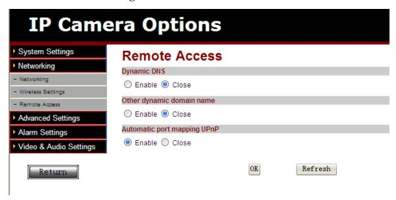
When remote access is needed, the dynamic DNS must be enabled, and fill the server address, server port ,username and password (the default server is user.ipcam.hk, the default server port is 808 . You can use the other dynamic DNS, such as peanut shell.
