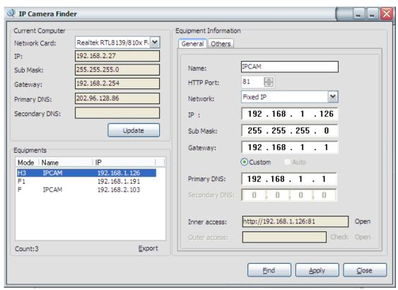
If network cable and power supply are correctly connected, device type, name and IP address will be shown in the device list (Otherwise, please confirm whether power supply and network cable work normally).
