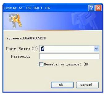
After selecting the language required, enter the corresponding log-in information, click ok to log in. Under the address bar, an ActiveX installation pop-up will appear. You can use it after installation. If the ActiveX intallation is held by the Anti-virus software, please release it.
