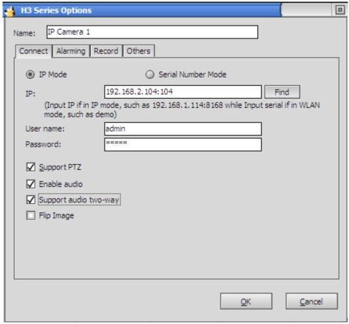
We can change the IP Camera name in the Super-Client. Select IP/domain mode or device code mode, If want to search the device in LAN mode, please click search. The search will be finished automatically. Then users need to input the account and password to view.
