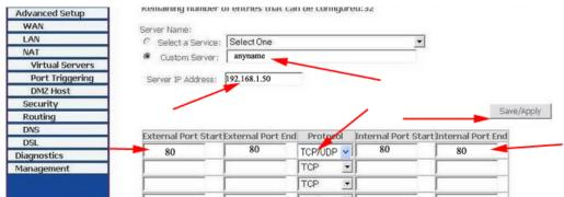
When complete port forwarding, you can visit camera through device code in outer net remotely;
