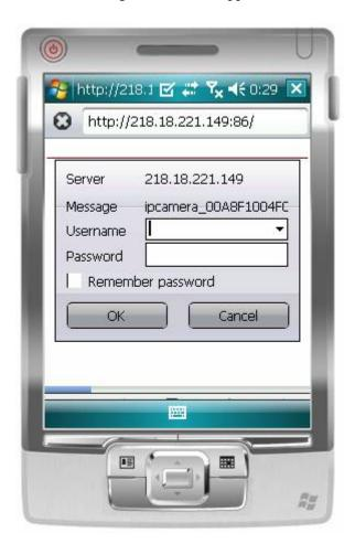
2.Input the Username and Passoword of the device, and the following interface will appear. There are three log-in options. Click on the third "Sign in" and use Mobile Phone mode.
