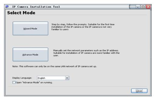
Wizard mode is remmended for primary users, open the IP camera and set device parmeters according to indication..
