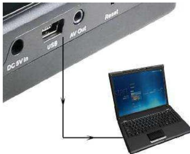
The default password is 00000 for connecting to PC. The DVR will be power off automatically when you disconnect the USB from PC.
