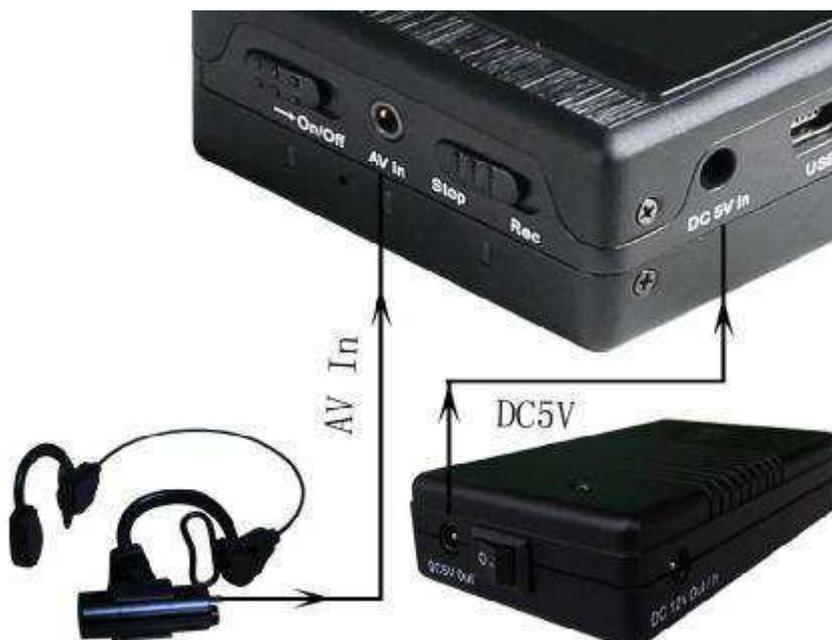
The UPS Battery Bank (7200mAH) can output DC 5V and DC12V voltage at the same time to power the DVR and a 12V Cameras for over 10 hours recording time, as shown in above Figure;
