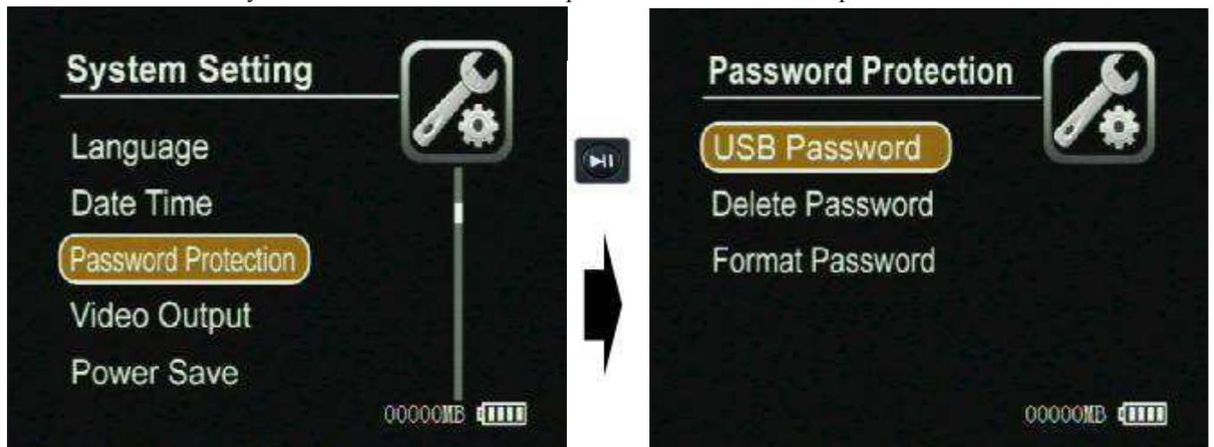
**USB Password:** You can set or enable or disable the USB password for accessing the DVR by USB.
